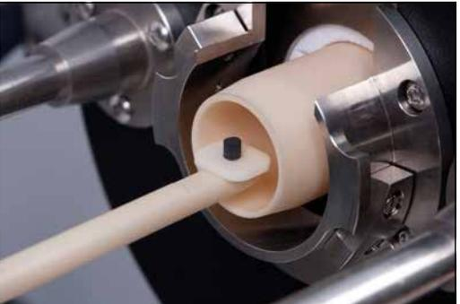
A detailed close-up photograph of a heating microscope. A light-colored, cylindrical sample is held within a complex metal chamber. A bright light source is directed at the sample, and a lens is positioned to observe it. The background is dark, highlighting the intricate mechanical details of the instrument.
