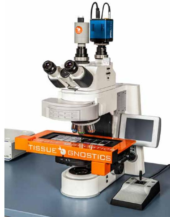
*TissueFAXS cytometers are highly flexible imaging and analysis platforms for IF/IHC processed samples*
